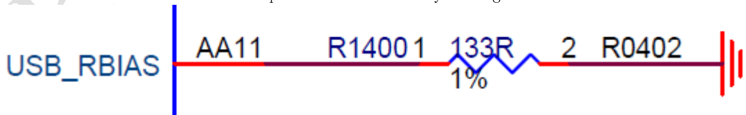
Figure 3-29 PX30 USB controller reference resistor
