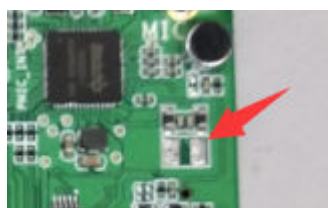
Figure 3-7 EVB speaker output
