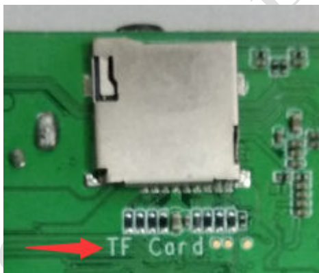
Figure 3-10 EVB TF socket
