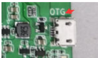
Figure 3-8 EVB USB OTG socket
