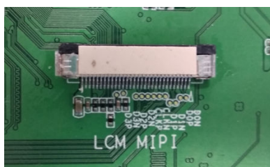
Figure 3-13 LCM-MIPI interface
