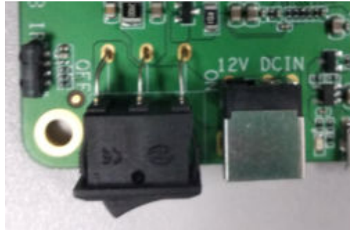
Figure 3-1 EVB power input
