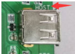
Figure 3-9 EVB USB HOST socket
