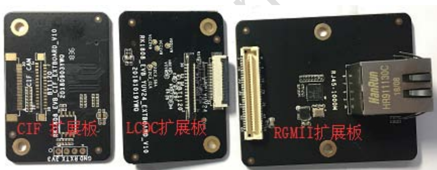
Figure 3-17 RGMII/LCDC/CIF extended small board
