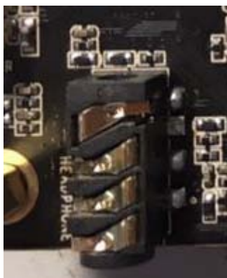
Figure 3-8 EVB audio input and output
