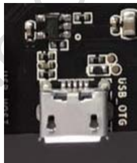
Figure 3-10 EVB USB OTG socket
