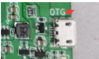
Figure 3-8 EVB USB OTG socket
