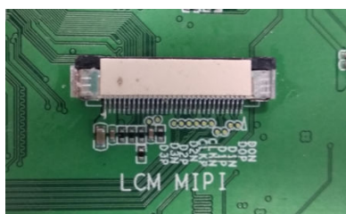
Figure 3-13 LCM-MIPI interface
