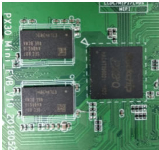
Figure 3-3 DDR3 location and physical picture
