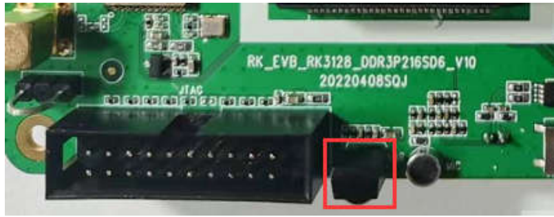
图 3-6 IR Receive 红外接收头
