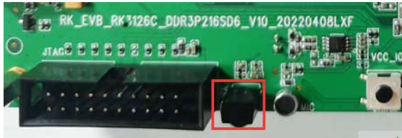
图 3-6 IR Receive 红外接收头
