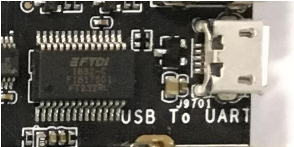
Figure 3-17 EVB UART debug port (USB Micro-B)
