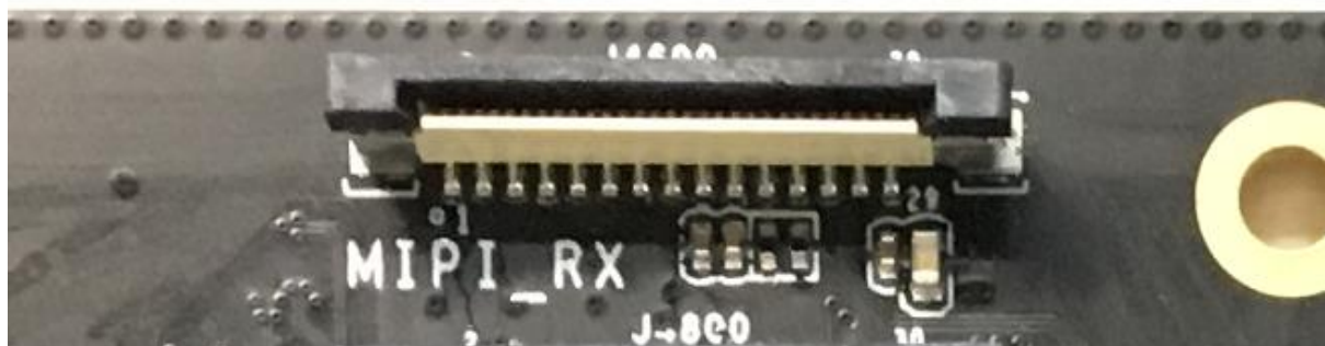
Figure 3-13 EVB MIPI camera connector
