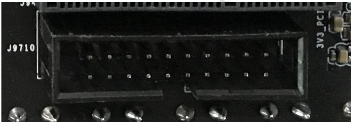
Figure 3-18 EVB JTAG debug connector
