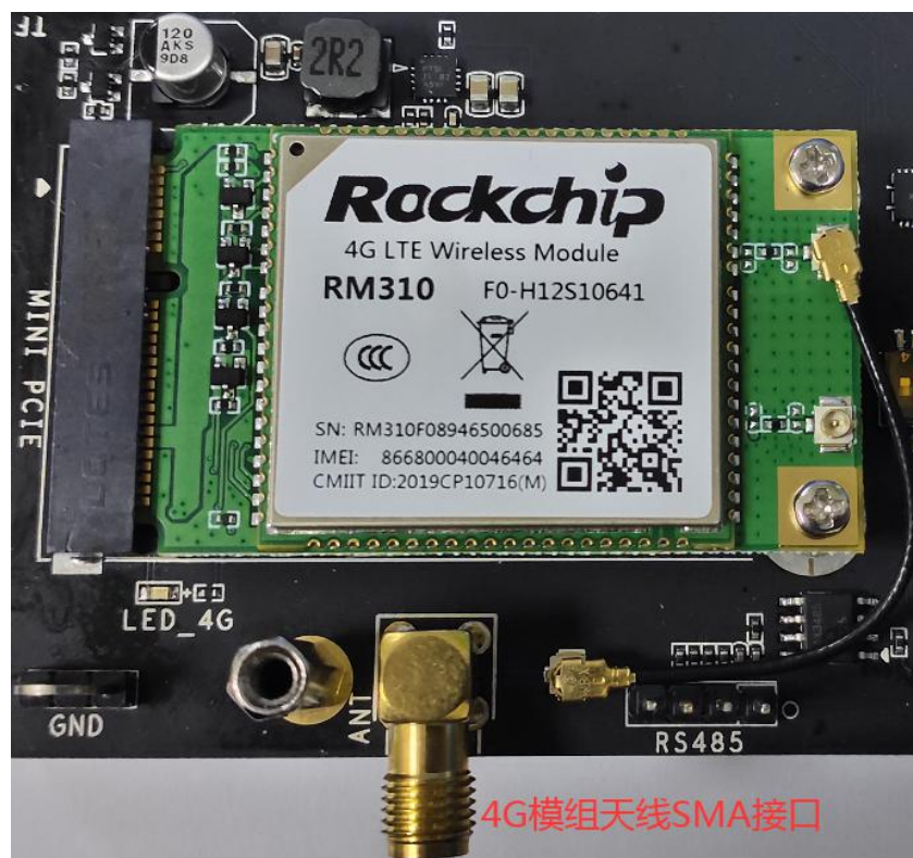
Figure 3- 33 4G module and antenna with SMA interface
