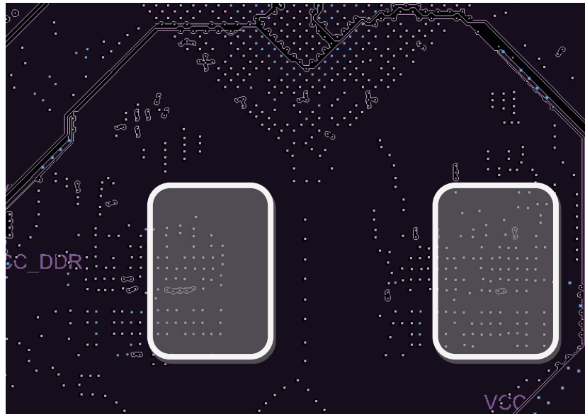
Figure 4-58 Reference Plane for DDR
