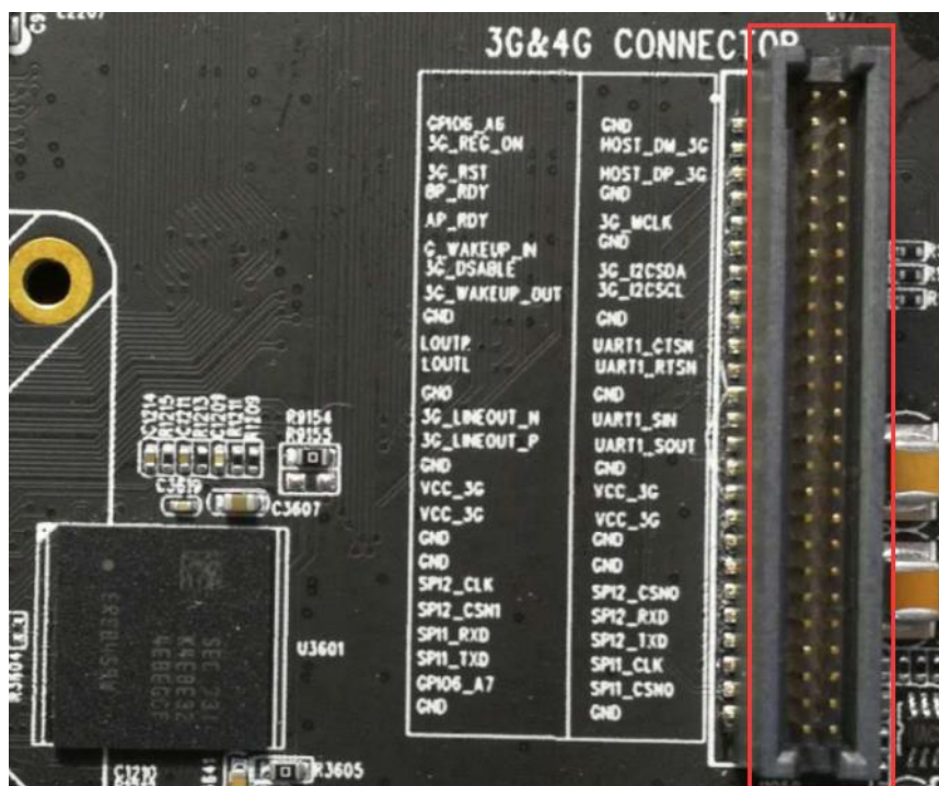
Figure 3-27 3G communication module extension Interface
