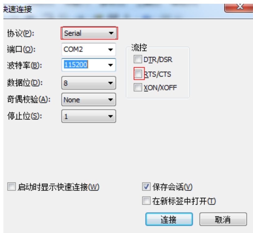
Figure 1-12 Configure serial port
