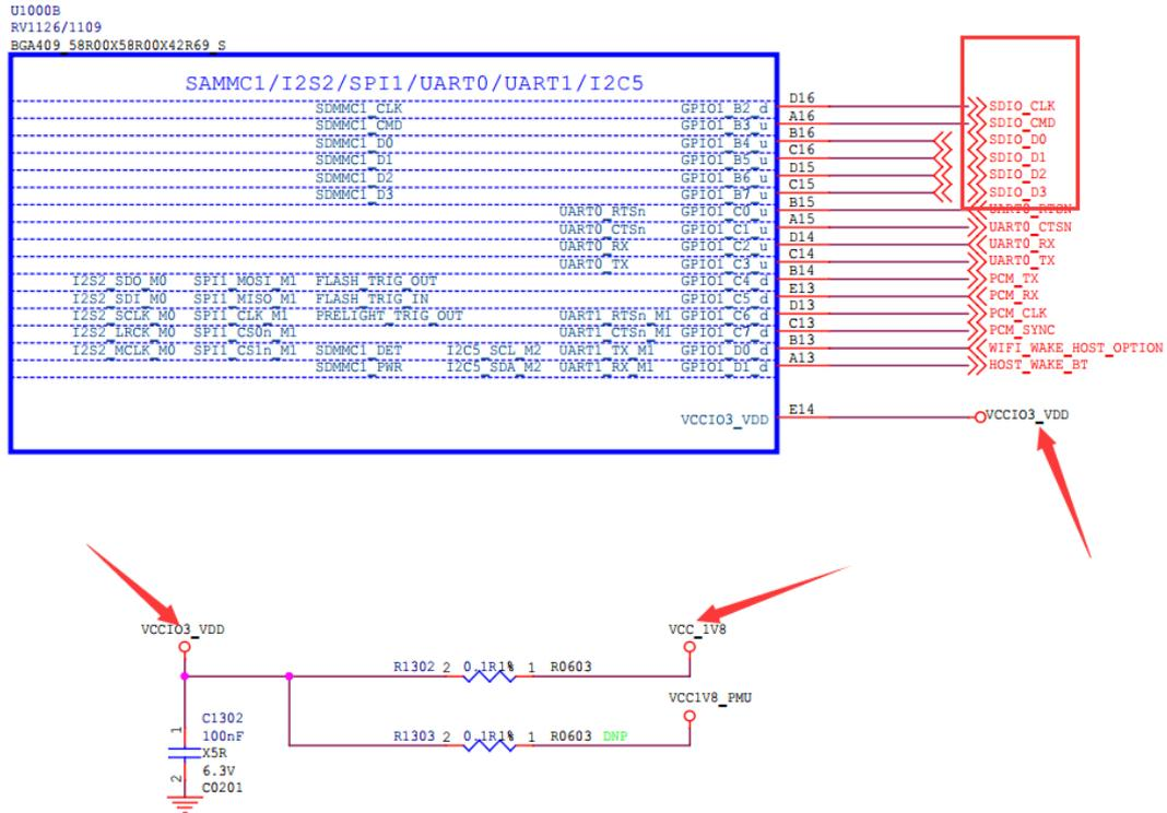
The other is the power supply of the IO of the Wi-Fi module. For example, the VCCIO\_WL in the figure below is also powered by VCC\_1V8. **The power supply of the two parts must be the same, otherwise it will lead to Wi-Fi abnormal;** for support SDIO3.0 Ultra-High speed Mode (UHS), it must be powered by 1.8V, but for Wi-Fi modules that only support SDIO2.0 high-speed mode, both power supply of 1.8 or 3.3V can be used, remember to keep matching ;
