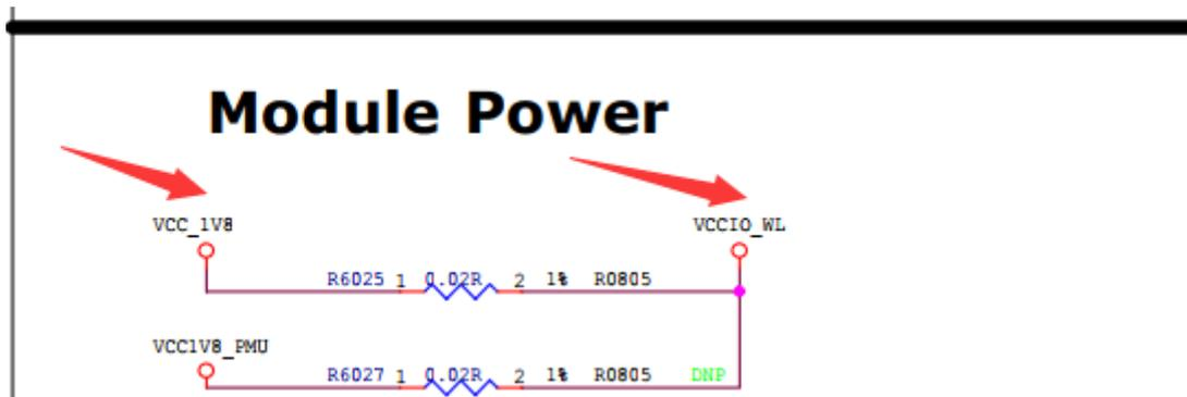
The above descriptions are all hardware requirements. The following is going to introduce the software configuration: From the above figure, it can be seen that the VCCIO3\_VDD supplying power to the controller IO is 1.8V, then the io\_domains corresponding to dts/dtsi need to be configured, and VDDIO3\_VDD corresponds to the software vccio3-supply, while vccio3-supply is powered by vcc\_1v8, the corresponding configuration is:
