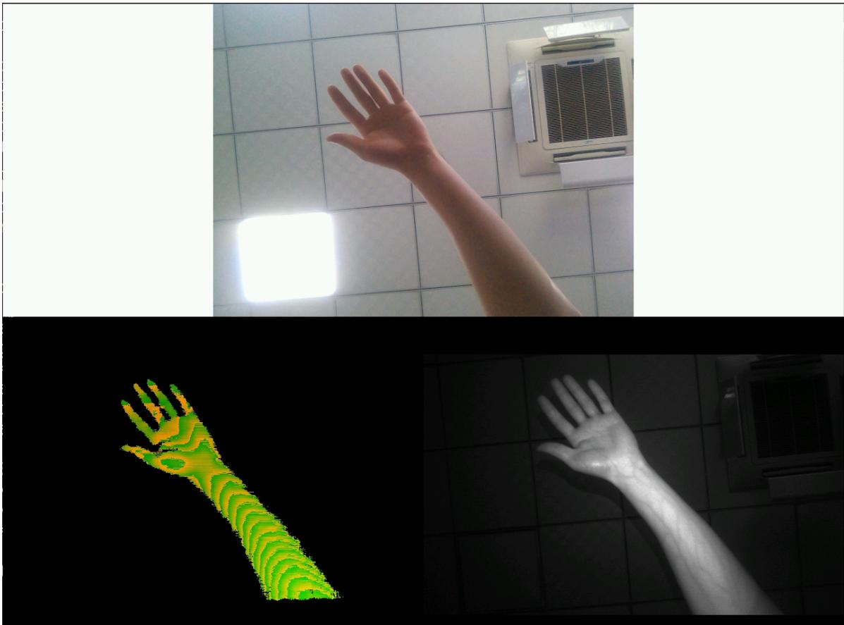
The pictures above show three images on RK3288 screen (1536x2048), from top to bottom and left to right, they are RGB, DEPTH, IR respectively. The size are all 640x480, in which the depth image displays the disparity image in RGB565 format directly.
